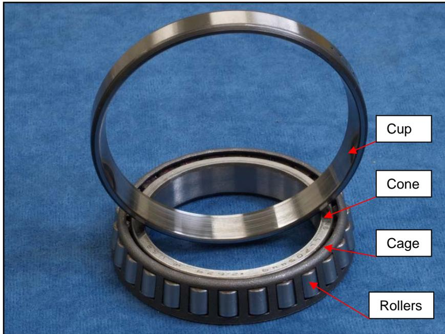
**Figure 7: Inboard bearing cone and cup**
